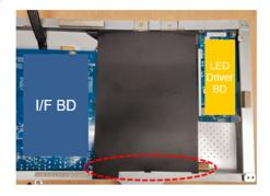
Unlock 10 PCBA screws to disassemble "I/F BD", "SPS BD" and "LED Driver BD" from Main SHD
