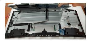
S16 Unlock 19 screws to disassemble Middle Frame from Panel
