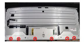
\$18 Disassemble Mylar from Main SHD
